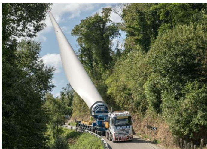
Figura 3 - Transporte de pás por blade lifter em vias estreitas ( https://trans.info/en/the-very-first-such-special-transport-in-spain-it-s-impressive-161955 ).
