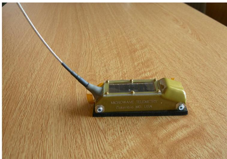
Figura 48 – Fotografia de PTT (Platform Transmitter Terminals)
